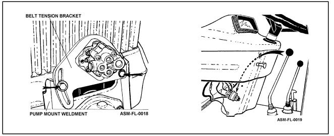
Remove ignition switch access panel or ignition switch if panels are not provided in dash. Identify the "Ignition-Start" wire and the "Ignition-Accessory" wire. **ASM-FL-0019**
